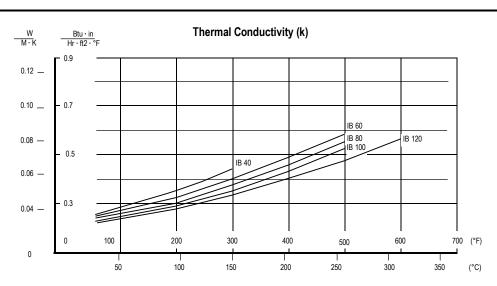
Based on measurements made in accordance with ASTM C-177 \* Steady State Heat Flux Measurements and Thermal Transmission Properties by Means of the Guarded Hot Plate Apparatus.
