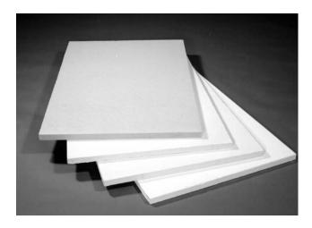
Superwool boards are processed from a slurry consisting of Superwool bulk and organic binders. Each board has cut edges for controlled squareness and trueness. Boards up to 36" wide may be ordered with both surfaces machined smooth to a close thickness tolerance.
