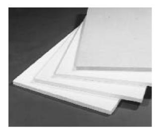
Superwool 607 PM boards are processed from a slurry consisting of Superwool bulk and organic binders. This board product is noted for its excellent surface finish, thickness uniformity and high insulating value at elevated temperatures.
