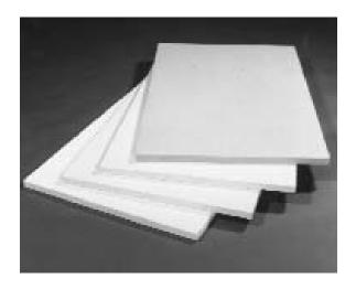
Thermal Ceramics vacuum formed products are a rigid self-supporting fiber insulation manufactured from a slurry consisting of Kaowool ceramic fibers and binders. Thermal Ceramics products have the capability to withstand chemical attack. Exceptions include hydrofluoric acid, phosphoric acid, and strong alkalies. A small amount of combustible binder will burn out at approximately 300°F. Additional hardness and strength can be achieved with post treatments.
