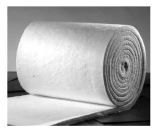
CER-WOOL blanket products are made from a spun process whereby as produced ceramic fiber is air-laid into a continuous mat and mechanically needled for added strength. CER-WOOL blankets do not contain organic binders and they are available in standard 24" and 48" widths and thickness from ½" to 2". Blanket strip in custom widths down to 3" wide can be made available to meet specific needs.
