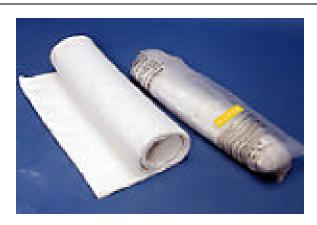
Cerafiber Wet Pack is manufactured by combining Cerablanket®, a needled refractory fiber blanket, and inorganic binding agents. Cerafiber Wet Pack is packaged in moist form in polyethylene bags. It is flexible and exhibits high tensile strength in the wet state. When air dried, it becomes a strong, hard, rigid structure.
